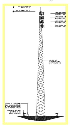
Pursuant to FAA regulations, the tower will be lighted with flashing red lights at night, and white strobe lights during the day.
